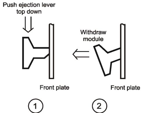
Figure 2: Function of the ejection lever
