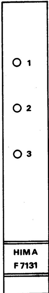
The module F 7131 monitors the system voltage 5 V generated by the 3 power supplies max. as follows:
