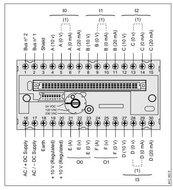
(1) For the current input unit, a jumper is required.
