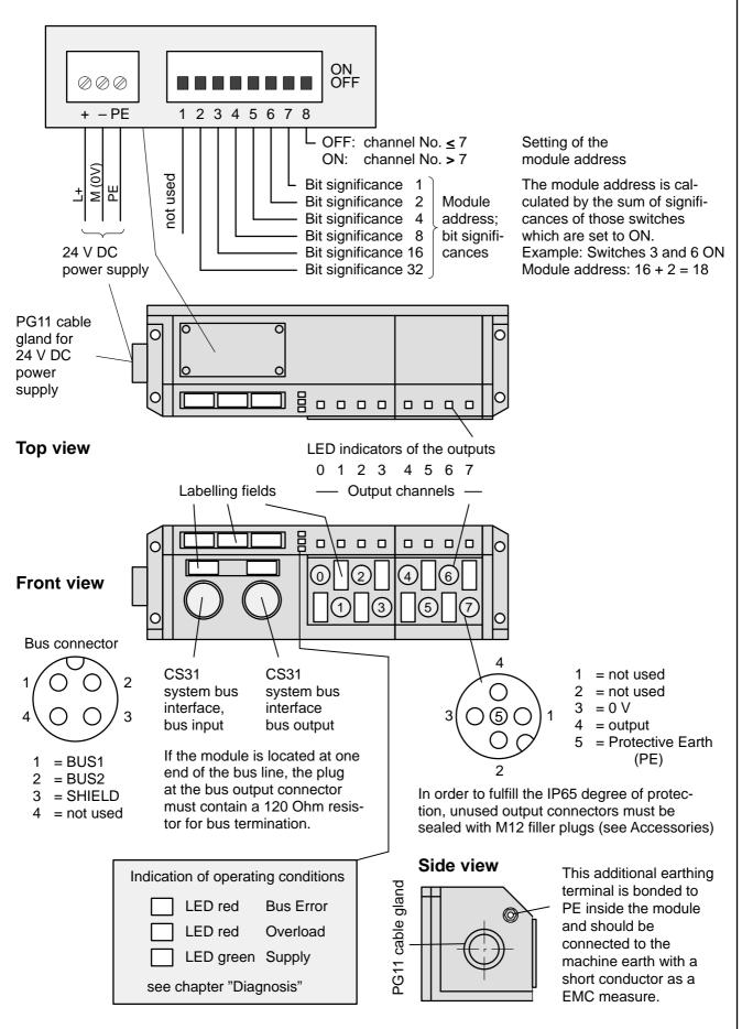
Fig. 4.4.2-2: Details for the electrical connection of the output module ICPO 08 H1
