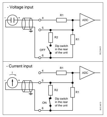
The wires for analogue inputs must be shielded and the shield has to be connected to the earth on the side of the remote unit.
