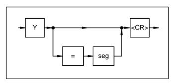
New segment address of the working segment seg: Keyword =:
