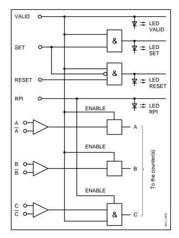
The input RPI enables the input C only for the modes 1, 2 or 3.
