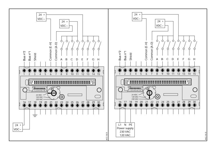
**Note** : In case of use of only one external power supply 24 VDC for inputs, the different communs have to be connected together and to the 0 VDC of the power supply.
