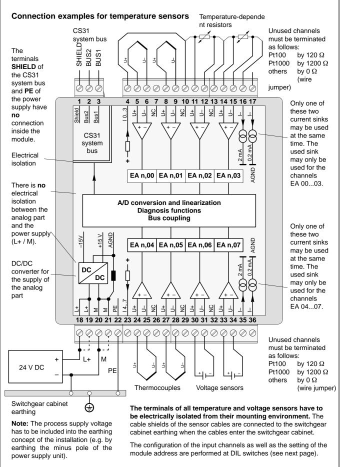
Fig. 5.2.5–2: Electrical connection of the analog input module ICDT 08 B5
