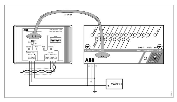
The 24 VDC power supply of the central unit can be used to supply only one unit NCC 485.
