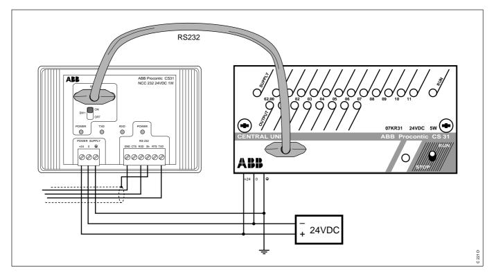
The 24 VDC power supply of the central unit can be used to supply only one unit NCC 232.
