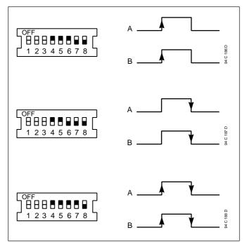
Impulses on input A count upwards, impulses on input b count downwards. Depending on the setting of the DIP switches, rising edges, falling edges or both edges trigger counting.
