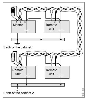
The capacitor is integrated in the plug-in base.
