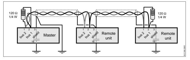
The bus must be terminated with a 120  $\Omega,$  1/4 Watt resistor, this must be connected at the ends of the bus.
