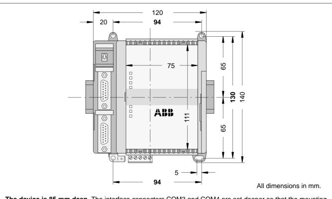
**The device is 85 mm deep.** The interface connectors COM3 and COM4 are set deeper so that the mounting depth required does not become any larger even with detachable interface cables. If, however, a DIN rail is used, the mounting depth is increased by the overall depth of the rail.
