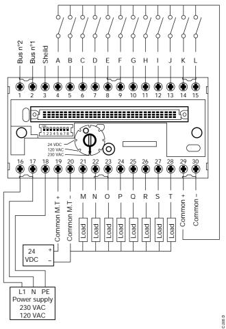
Electrical schema for an output
