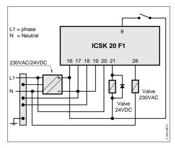
Example of connection with a 230 VAC power supply
