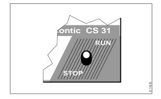
The **RUN/STOP** switch is used to start or abort the processing of the user program.
