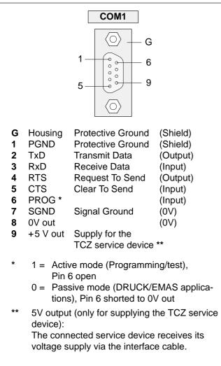
Fig. 1–15: Assignment of the serial interface COM1
