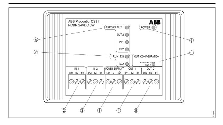
The NCBR is an amplifier for CS31 bus with integrated redundancy functions.
