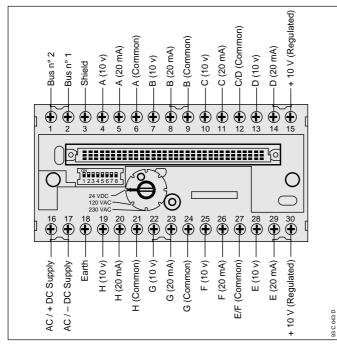
The function of each channel depends on the wired terminals.
