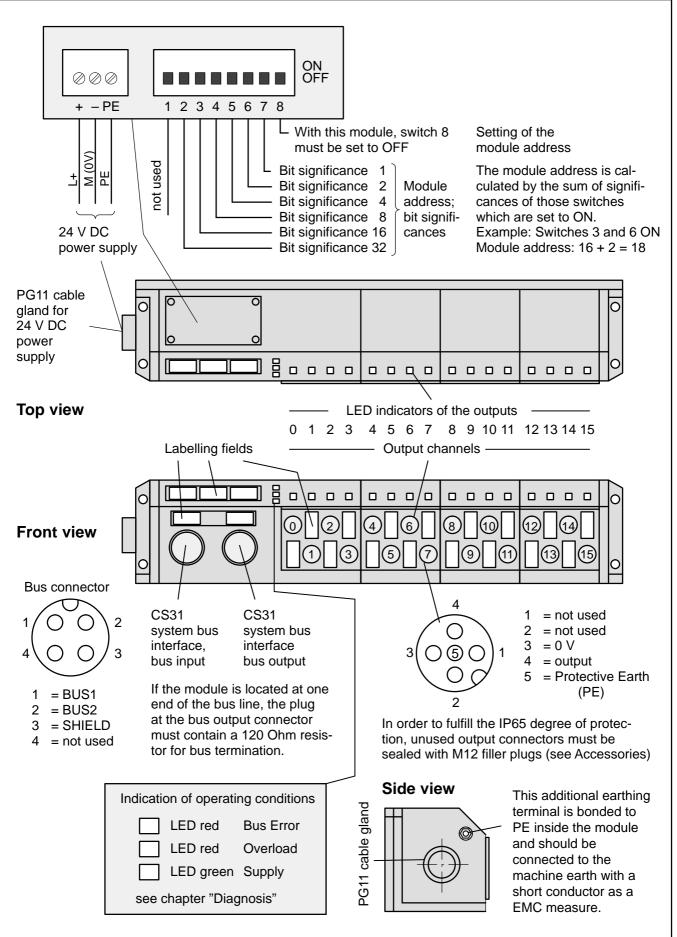
Fig. 4.4.1-2: Details for the electrical connection of the output module ICPO 16 H1
