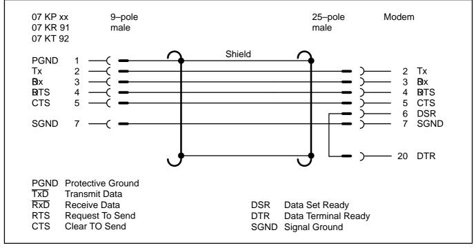
Fig. 13.8.4–2: Terminal assignment of 07 SK 92
