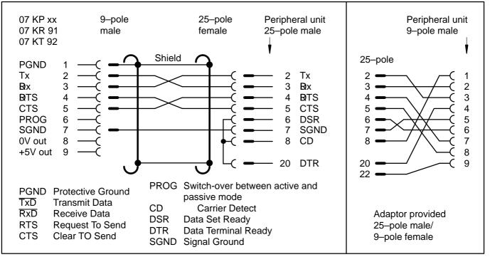
Fig. 13.8.2-2: Terminal assignment of the 07 SK 90 interface cable and the adaptor provided with
