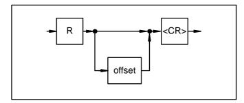
offset: Offset (by addition to the segment address of the address extension record, this results in the new segment address)
