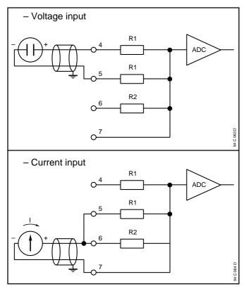
The wires for analogue inputs or output must be shielded and the shield has to be connected to the earth on the side of the remote unit.
