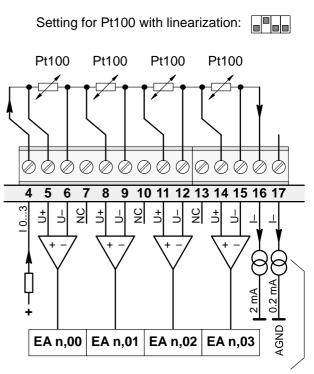
Only one of these two current sinks may be used at the same time. The used sink may only be used for the channels EA 00...03.
