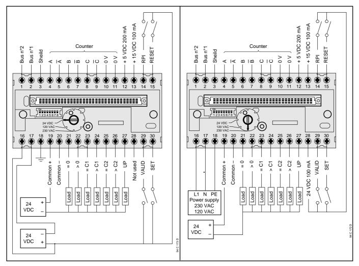
**Note** : When using the 230 VAC or 120 VAC versions, the internal 24 VDC supply can be used providing the load if it is not greater than 50 mA; if it is, an external 24 VDC power supply must be used.
