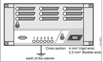
Example of connection with a 24 VDC power supply
