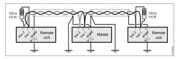
When noisy elements are in the area of the cabinet, it is better to connect the bus' shield to the ground via a capacitor 1 nF class Y directly at the access of the cabinet according the following diagram.
