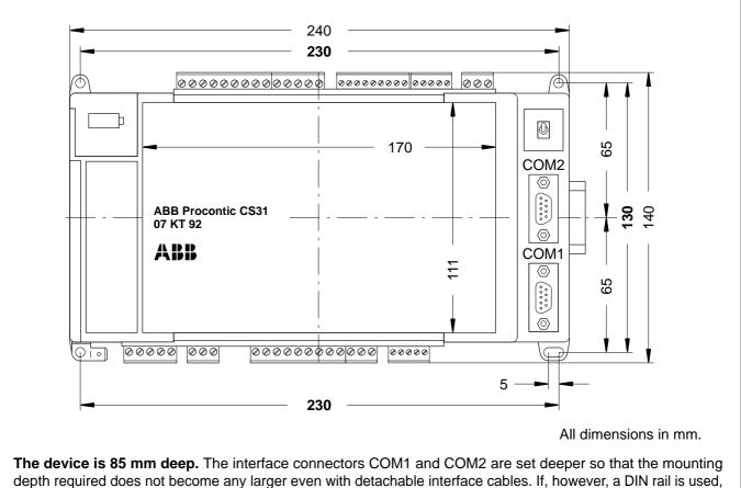
the mounting depth is increased by the overall depth of the rail.
