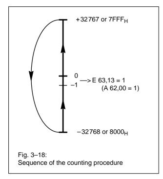
• Enabling/disabling of the counting procedure using the internal variable A 63,14 in the user program:
