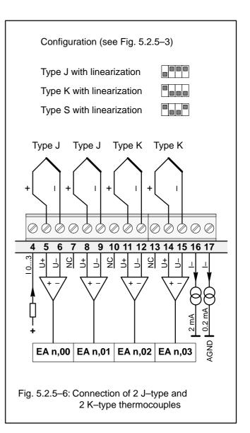
The thermoelectric voltage generated by the thermocouples is converted into binary values inside the module and then linearized according to the thermocouple type. In order to get the absolute temperature, the temperature of the reference junction is added.
