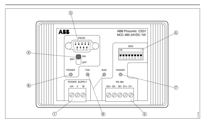
The NCC 485 module is an RS232/RS485 interface converter. It is the solution of transmission problems in industrial data communications.
