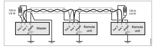
The bus must be terminated with a 120 , 1/4 Watt resistor, this must be connected at the ends of the bus. The central units UCZA/UCZB, the couplers 07 CS 61 and 35 CS 91 have to be connected at an end of the bus. The resistor 120 is integrated.
