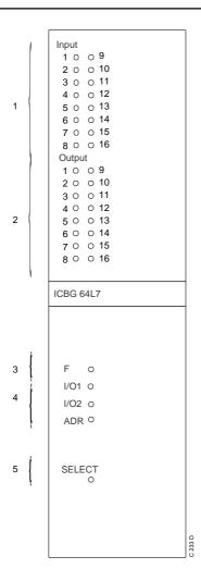
Robot coupler 64 Inputs/Outputs
