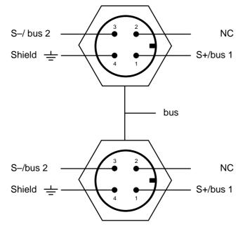
Fig. 12.2–2: Connection on the field bus node
