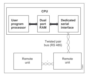
In the read cycle, data is taken from the remote unit and stored within the dual port RAM via the bus and dedicated serial interface, the user program processor then reads the data from the dual port RAM.
