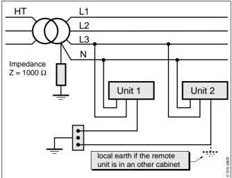
In a noisy environnement, an isolated transformer with a shield has used in each cabinet (even for 24 VDC version).
