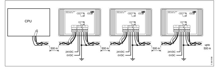
The resistance for end of line (120  $\Omega$  1/4W) is already integrated into the NCB.
