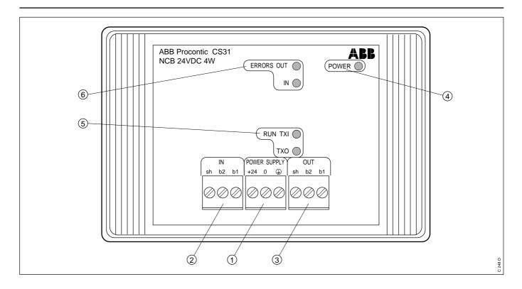
The NCB is an amplifier for CS31 bus. It ensures a amplifier function whereas the maximum lenght on one bus can reached upto 2km with the installation of 3 NCB.
