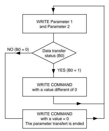
Before using a new command (to send new parameters), the value 0 has to be loaded in the command word.
