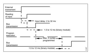
The bus transmission time is easily calculated from the configuration of the installation.
