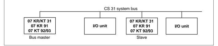
Without regard to the address ranges, the following units can be connected to a CS31 system bus :
