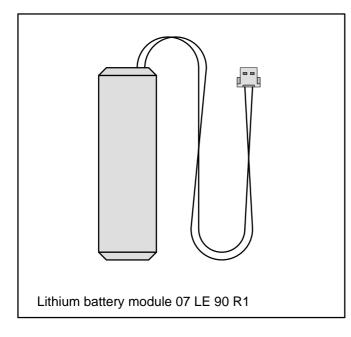
The 07 LE 90 R1 lithium battery module is used for RAM data back-up in several processor units of ABB Procontic programmable control systems. In order to change the battery quickly, it is equipped with a 2-pole plug and two soldered wires.
