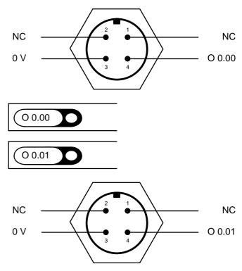
Fig. 12.2–4: Connections for additional outputs
