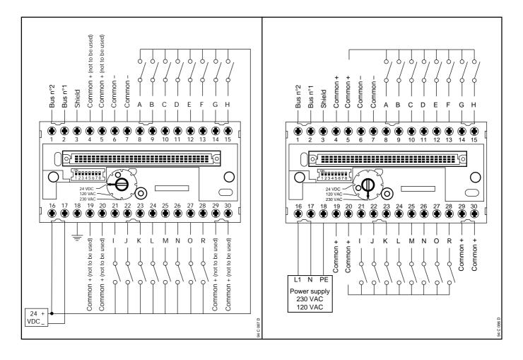
Note : In case of use of an external power supply 24 VDC for inputs, the "0" VDC has to be connected to the common "-".
