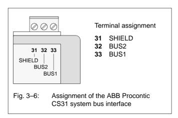
The connection to the ABB Procontic CS31 system bus is made by means of a 3-pole detachable terminal block. Please observe:
