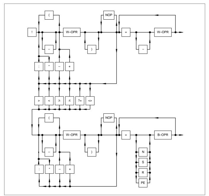
Signal flow:in direction of arrow, otherwise from left to right.Brackets:sum "LEFT BRACKET" = sum "RIGHT BRACKET", nesting depth: 15.W-OPR:Word operand (EW, AW, MW, KW)<br/>Example: EW 03,05 AW 11,12 MW 22,15 KW 09,06B-OPR:Binary operand (E, A, M, S, K)<br/>Example: E 00,03 A 07,06 M 05,01
