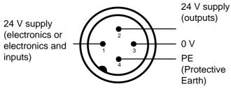
Fig. 12.2–3: Connections for 24 V supply
