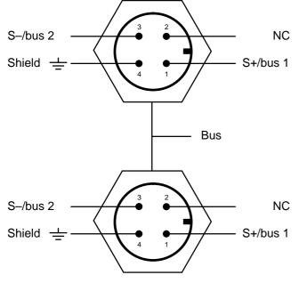
Both socket-outlets are internally wired in parallel.
