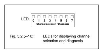
When releasing the test button, the error information belonging to this channel is displayed by the green LEDs 0 to 7 for a period of ca 3 seconds.
