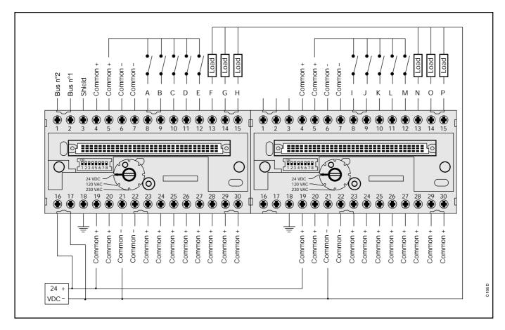
**Note :** Almost one common + and one commun – on each plug-in base ECZ have to be connected to the power supply.
