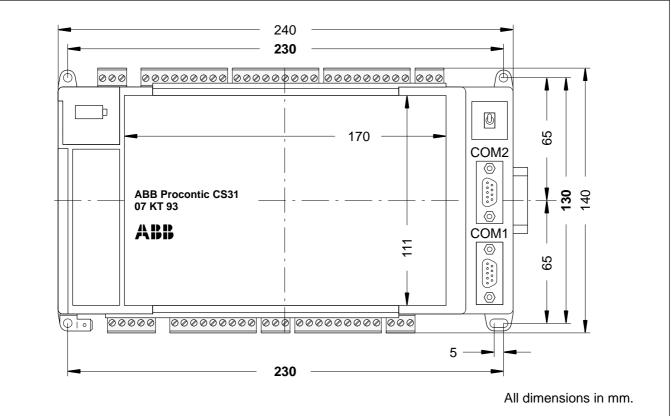
**The device is 85 mm deep.** The interface connectors COM1 and COM2 are set deeper so that the mounting depth required does not become any larger even with detachable interface cables. If, however, a DIN rail is used, the mounting depth is increased by the overall depth of the rail.
