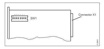
Insert the card into a binary input/output slot of the robot rack (refer to robot documentation for user details).
