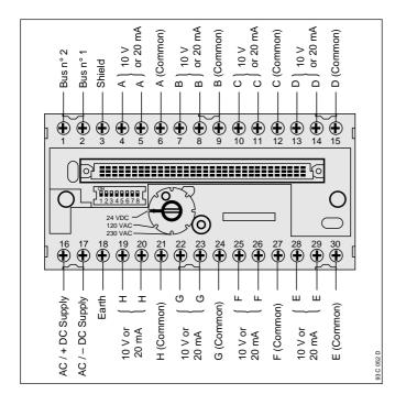
NOTE : All common terminals are internally connected but it's better to use the terminal nearest the channel used.
