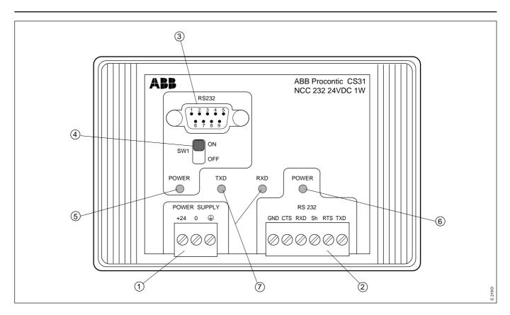
The NCC 232 module is an RS232/RS232 interface converter. It is the solution of transmission problems in industrial data communications.
