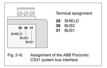
The connection to the ABB Procontic CS31 system bus is made by means of a 3-pole detachable terminal block. Please observe:
