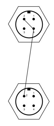
Fig.12.2–5: Connections for signal inputs
