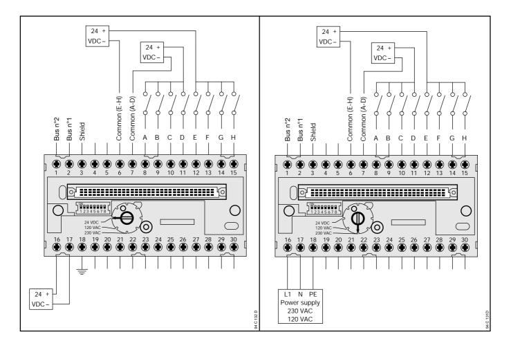
Note : In case of use of an external power supply 24 VDC for inputs, the "0" VDC has to be connected to the common "–". Caution : The 24 VDC must never be connected to
