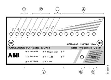
4 analog inputs and 2 analog outputs per unit
