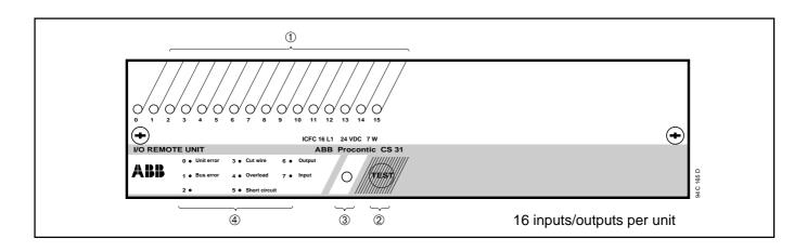
Binary input/output unit with 16 channels.
