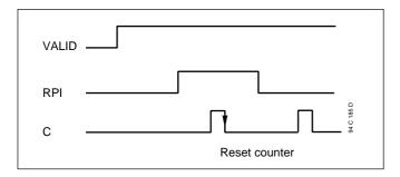
The falling edge of C resets the counter to 0 while RPI is ON. The signal C must not occur twice or more times within one period of RPI. The VALID must be ON.
