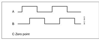
The above shown pulse diagram results in counting upwards. The counting direction can be reversed by interchanging inputs A and B.
