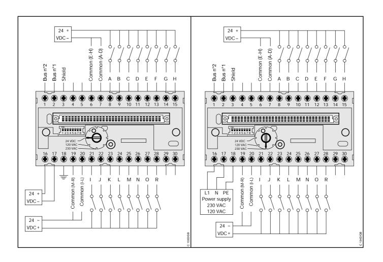
**Note** : In case of use of only one external power supply 24 VDC for inputs, the different communs have to be connected together and to the O VDC of the power supply.
