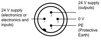
Fig.12.1–3: Connections for 24 V supply
