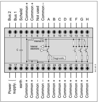
Note : In case of use of an external power supply 24 V DC for inputs, the "24" V DC has to be connected to the common "+".
