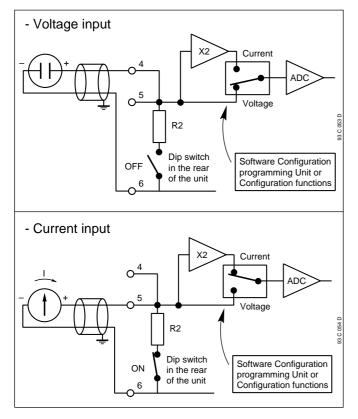
The wires for analogue inputs must be shielded and the shield has to be connected to the earth on the side of the remote unit.
