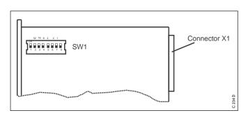
Insert the card into a binary input/output slot of the robot rack (refer to robot documentation for user details).
