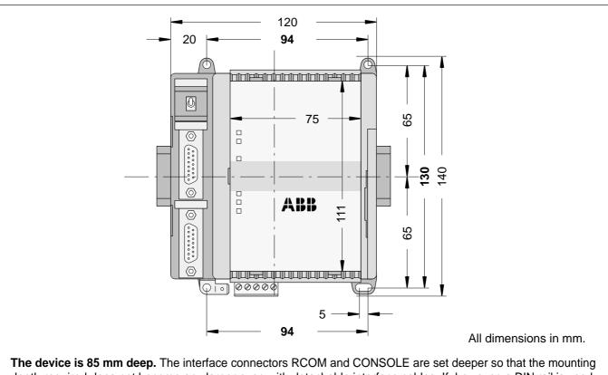
**The device is 85 mm deep.** The interface connectors RCOM and CONSOLE are set deeper so that the mounting depth required does not become any larger even with detachable interface cables. If, however, a DIN rail is used, the mounting depth is increased by the overall depth of the rail.
