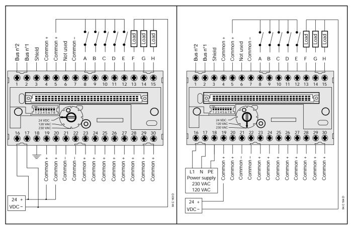
**Note :** Almost one common + has to be connected to the power supply. When switching high current loads, use many commun + terminal to avoid damage to the base.
