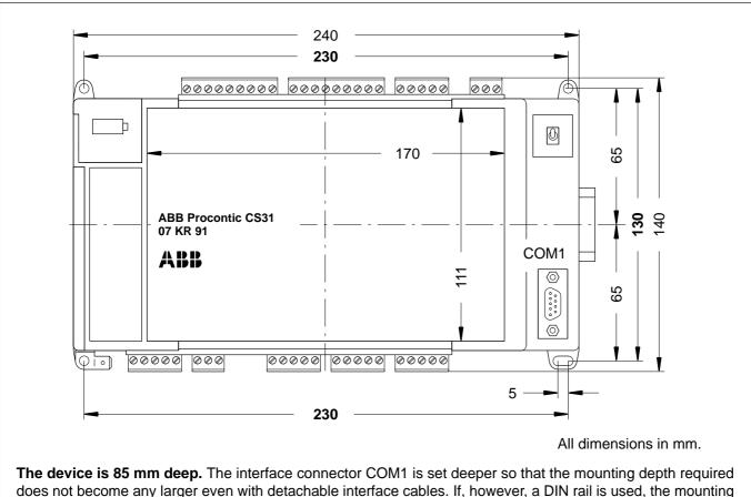
does not become any larger even with detachable interface cables. If, however, a DIN rail is used, the mounting depth is increased by the overall depth of the rail.
