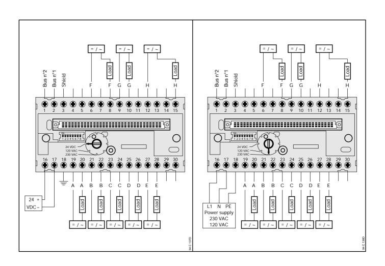
**Note** : In case of inductive load with a DC current, a free wheele diode Has to be mounted in parallel of the load according the following example for the output A :
